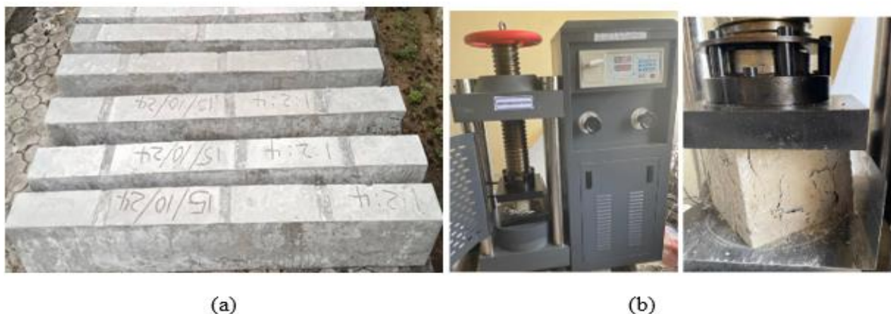
Plate 1: (a) RC Beam; (b) Universal Compression Machine
