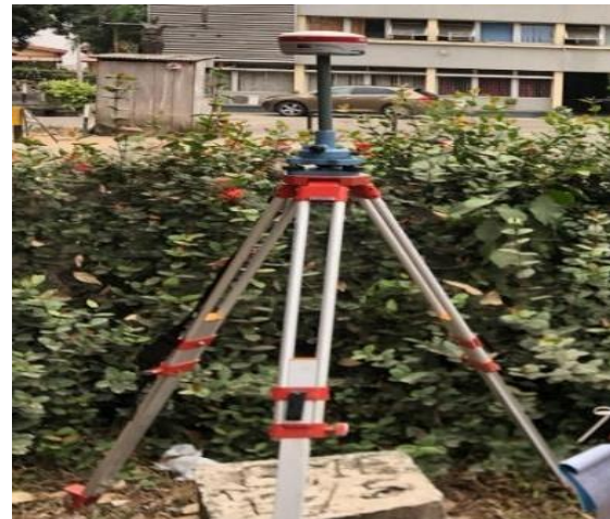
Figure 4: Stonex S900A Setup on GME 17/5
