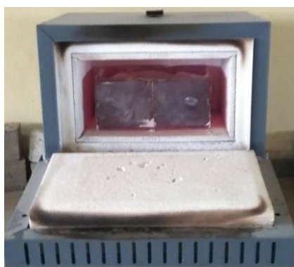
Figure 2: Calcination process of kaolin
