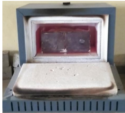
Figure 2: Calcination process of kaolin
