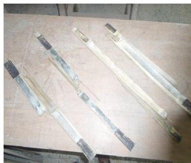
Figure 6: Failure patterns of bamboo specimens.
