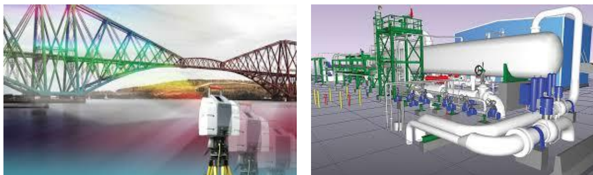
Figure 4: Application of laser scanner on bridge and pipeline (Source: Mills et al., 2004)
